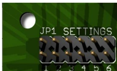
JP1 is used for general configuration like PARALLEL or BINARY interface, and Nayax Counter signal length and value.
