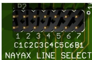
JP2 is an integrated PULSE adapter to convert the Nayax PULSE signal to the corresponding COIN #1- #6 or BILL #1 line to connect.
