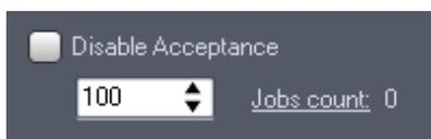
Disable cash acceptance if jobs counter reaches this setting. For example the machine has 100 sheet of paper, set this trigger to 100 and reset the jobs counter. If the jobs counter reaches this trigger, we do not accept money anymore.
