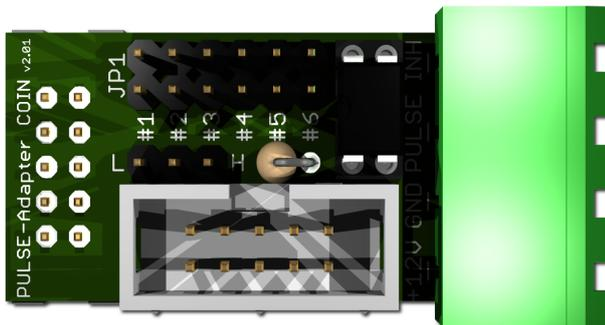
The [PULSE-Adapter COIN](#) has a 10 pin connector that fits to default coin plugs, and offers again a 10 pin coin plug to plug in the originally coin acceptor cable, so you do not lose the coin acceptor connector. The cashless device can be connected easily via plugable terminal connector. With a jumper you can select the coin channel on which the external credit signal is transferred.
