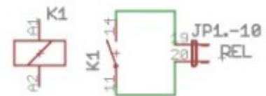
As you can see the push button must be connected to IN1. Use one of the included 2 pin cables and plug it on the IN1 pins (pin 9 and 10), then extend that 2 wires for your needs to the push button itself. On the push button you see COM and NO inscription, same on the schematic.
