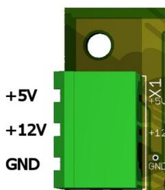
The power supply is connected to terminal plug X1.
