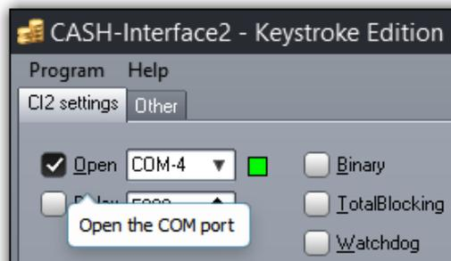
The connection to the CASH-Interface2 is open now and commands can be sent and data received. When the COM port is opened, the CASH-Interface2 sends all stored settings to the PC. You can see that in the log file if "log all" is activated.
