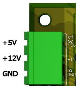
The power supply is connected to terminal connector X1.
