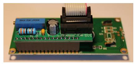
The manufacturer of the LCD display suggests to NOT use flat ribbon cables longer than 10cm to avoid display problems by interfering signals! If you use longer cables and get problems change to a shorter cable length or use an shielded cable.
