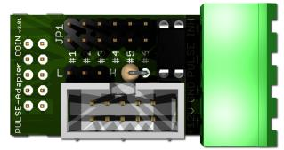
The **PULSE-Adapter COIN** has a 10 pin connector that fits to default coin plugs, and offers again a 10 pin coin plug to plug in the originally coin acceptor cable, so you do not lose the coin acceptor connector. The cashless device can be connected easily via plugable terminal connector. With a jumper you can select the coin channel on which the external credit signal is transferred. Additionally there is
