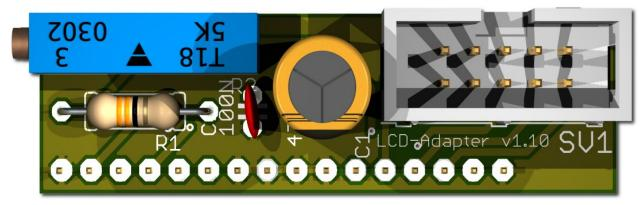
Depends on the used LCD display, the adapter has to be mounted on the left or right side. Some displays have the power pins on the left side others on the right side! Hint: since version 1.10 the LCD-Adapter only
