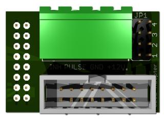
The **PULSE-Adapter BILL** has a 16 pin connector that fits to default NV9/NV10 plugs, and offers again a 16 pin plug to plug in the originally bill acceptor cable, so you do not lose the bill acceptor connector.
