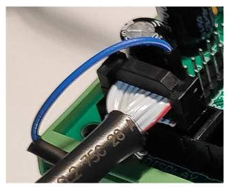
For the grounding of the cable shielding, the shielding is carried out on one side with a single dupont cable with an female connector, and can therefore simply be plugged onto GROUND (JP2 - GND) on the CI MC8 circuit board.
