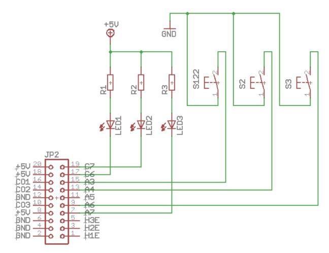
To illuminate the buttons there should be LEDs used because they need less current. Every output can supply 500mA, for higher current use an external relays. If you use a relays, be sure to add a freewheeling diode to the relays coil, or the output on the CI MC8 gets destroyed!
