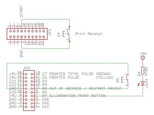
The PRINTER PULSE output is an OPEN COLLEKTOR Output, with max. 500mA current (ULN2803). Instead of a printer it is possible to connect an external counter or hard meter. If a relay is used, a free-wheeling diode must be connected parallel to the relay coil, otherwise the output will be destroyed!
