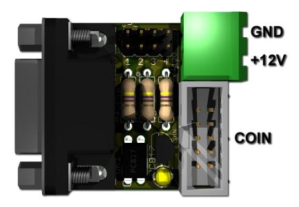
Hint: The coin validator MUST work with PULSE protocol, because the adapter just monitors output line 1!!!
